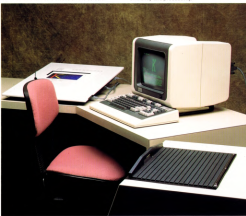
(Left, Centre) Broken or irregularly formed characters are highlighted on the system's screen to assist the operator in verifying identification. Users can also edit text as it scrolls on the screen.
